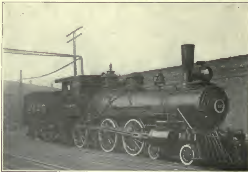
FIG. 380. LOCOMOTIVES Passenger Locomotive of the Ten- wheel Type. Chicago, Milwaukee & St. Paul Railway.
